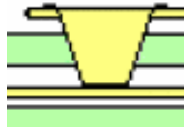
A Micro-via showing a tapered hole
